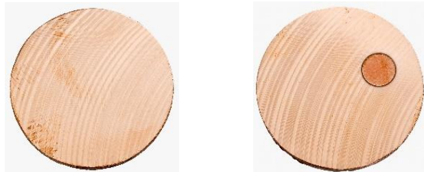
Metallic disc before and after GD-MS measurement.
