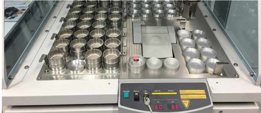
Sample chamber of WD-XRF (4 KW), Axios, Panalytical
