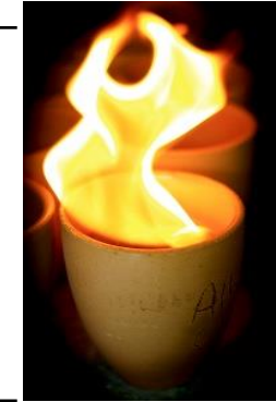
Crucibles in furnace for fire assay at (1000 - 1100°C).
