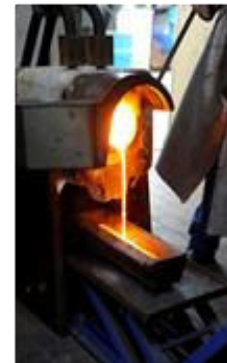
pouring melted sample into a casting mould
