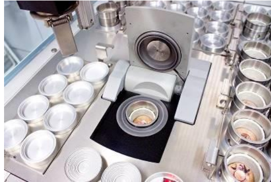
Sample chamber of WD-XRF (4 KW), Axios, Panalytical
