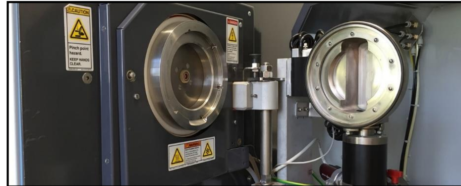
Sample chamber with ion source in GD-MS PLUS.
