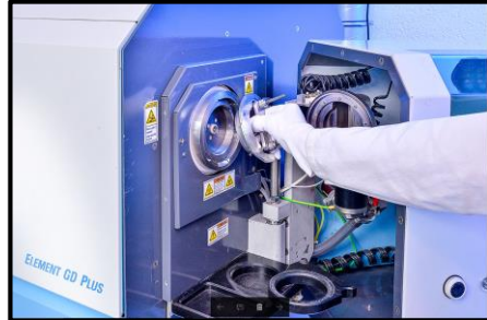
Sample mounted in ion source
