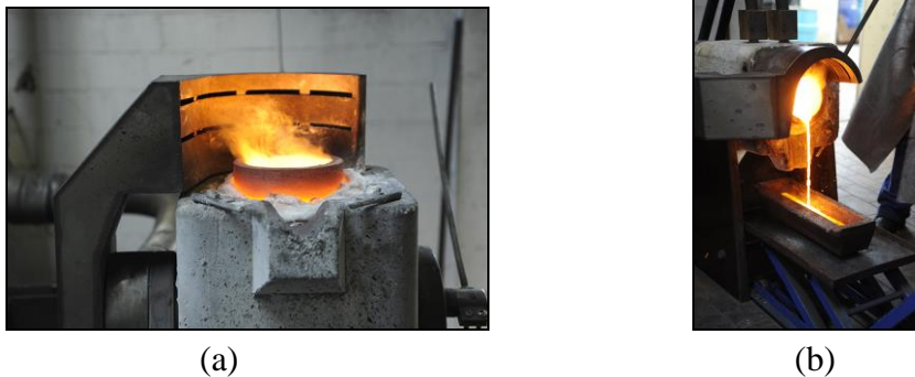
Figure 2. (a) Melting the sample mixture in an induction furnace and (b) casting for further treatments for sample preparation at IMG, Willich.
