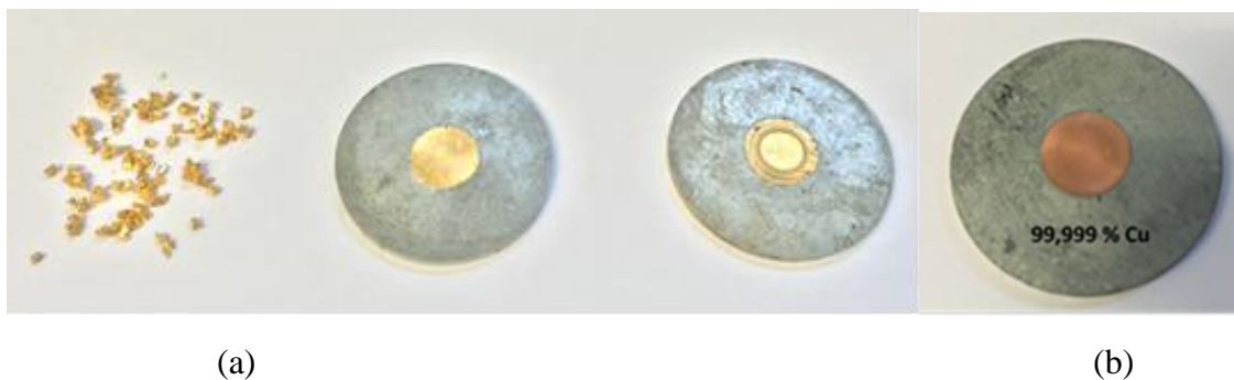
Figure 11: Presslings from (a) gold granulates and (b) copper powder in steel discs for GD-MS measurement.
