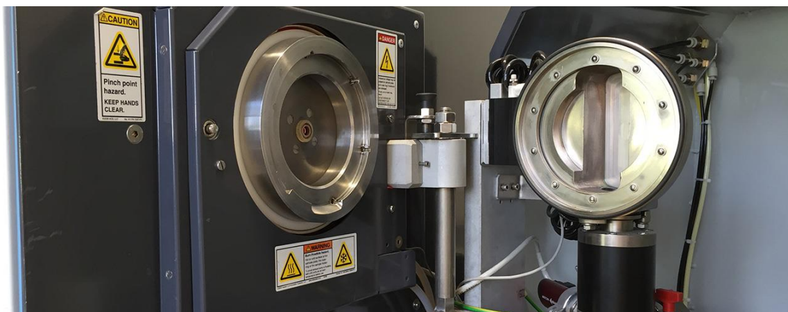
Figure 9. Sample chamber with ion source in GD PLUS GD-MS.
