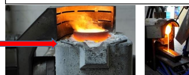
Induction furnace and casting mould
